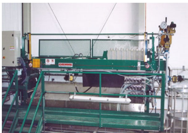
Membrane Filter Press 8.19 m2 (Plates 630 x 630 mm)
