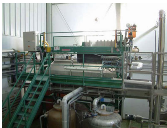
Membrane Filter Press 8.19 m2 (Plates 630 x 630 mm)
